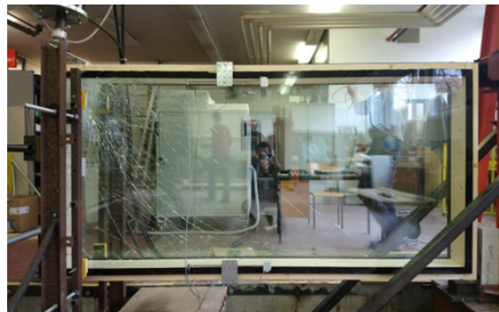
Figure 2: Presentation of the fracture mechanism of the timber DSF wall element in experimental testing.
