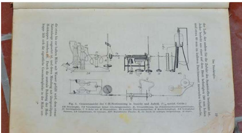
Schematic representation of the original device for the determination of carbon and hydrogen in the organic compounds in mg quantities. For this method Frederick Pregl, chemist of Slovenian origin received the *Nobel Prize in 1923*. The scheme on the photo is shown in the book of Friderik Pregl issued in 1916. (page 22)
